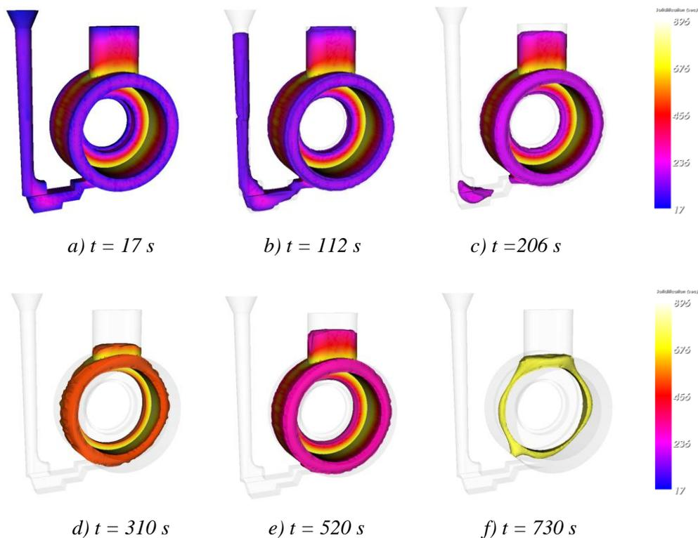
Figure 5. The solidification process of the casting.
