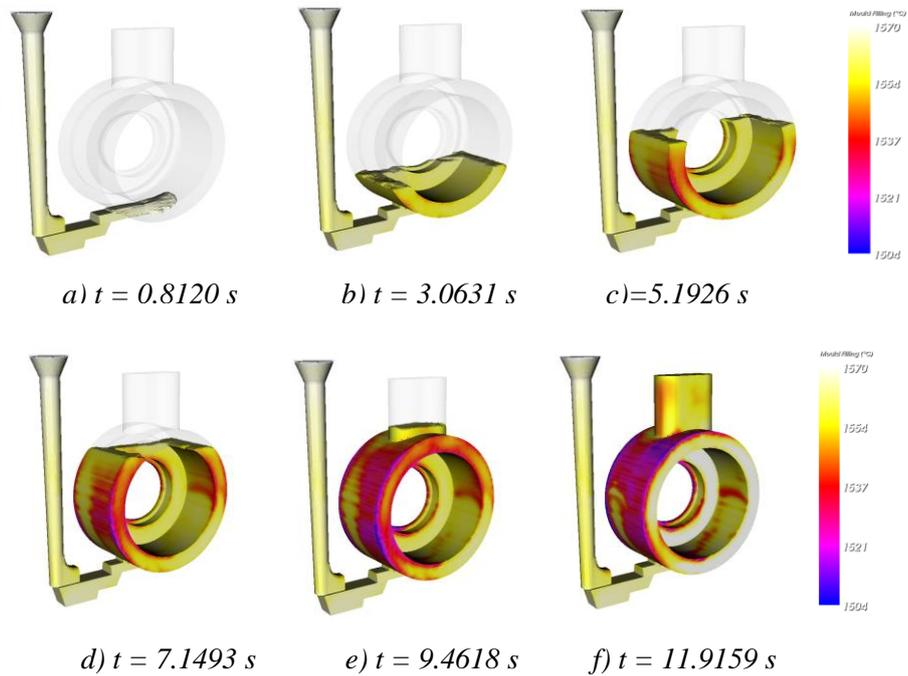
Figure 6. Mould-filling process of the casting technology.
