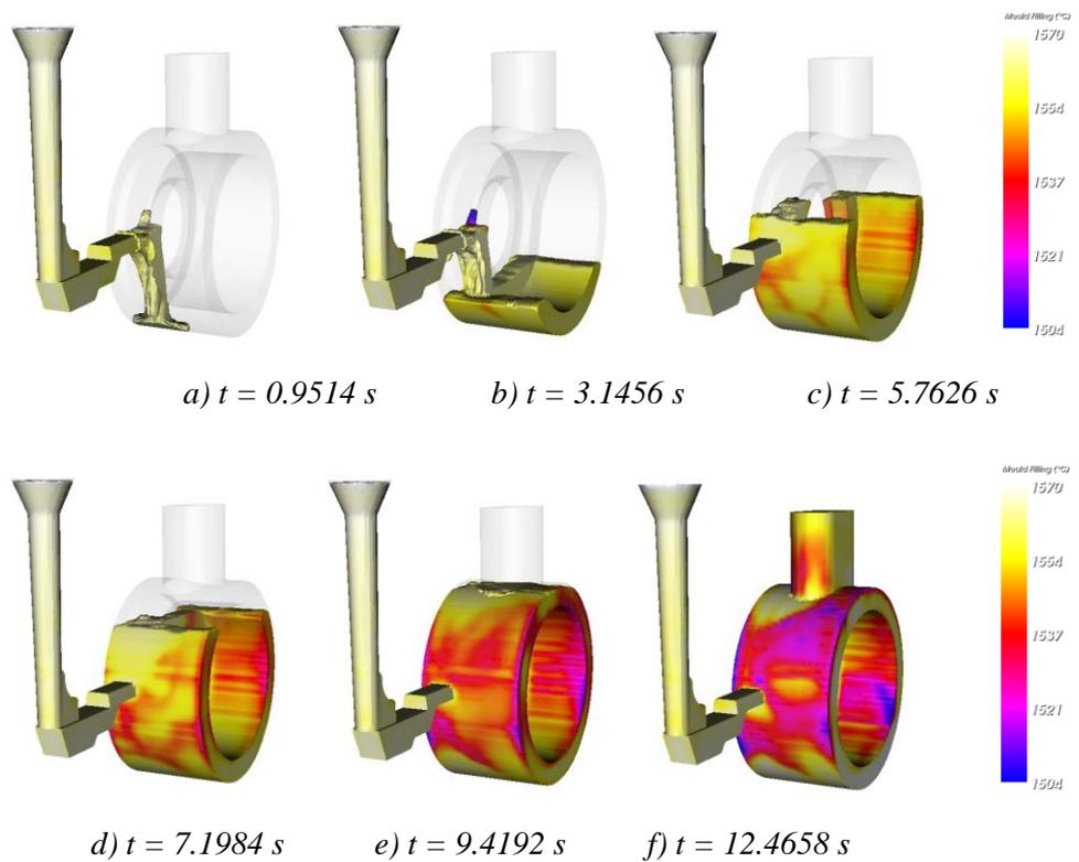
Figure 9. Mould-filling process of optimized scheme I.
