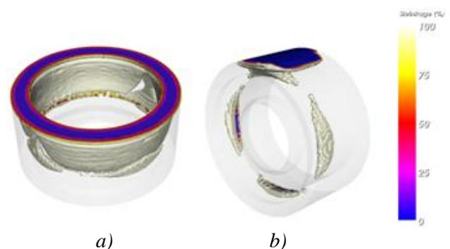
Figure 2. Defect forecast map of the sleeve:
