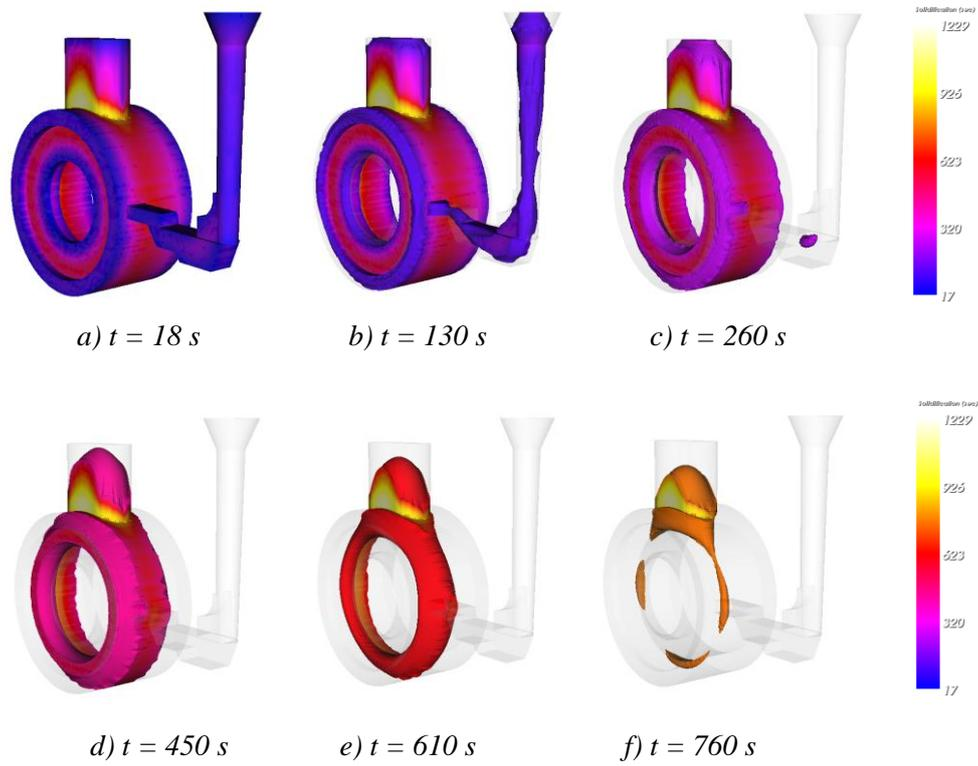
Figure 8. The solidification process of optimized scheme I.
