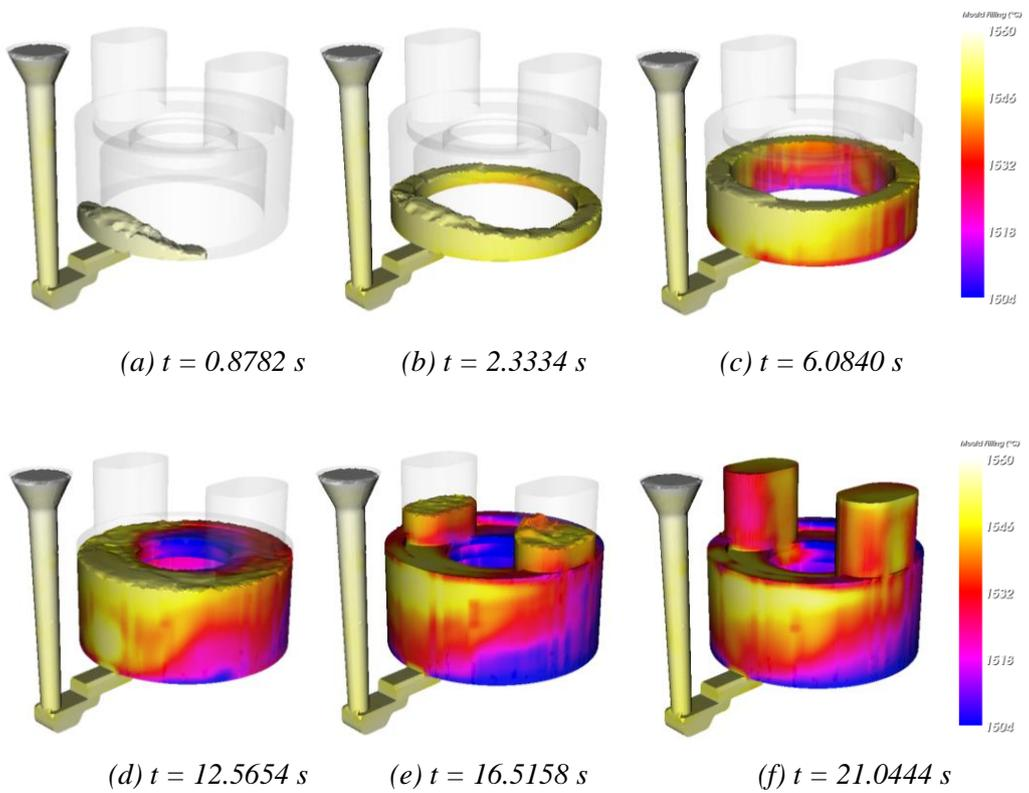
Figure 11. Mould-filling process of optimized scheme II.
