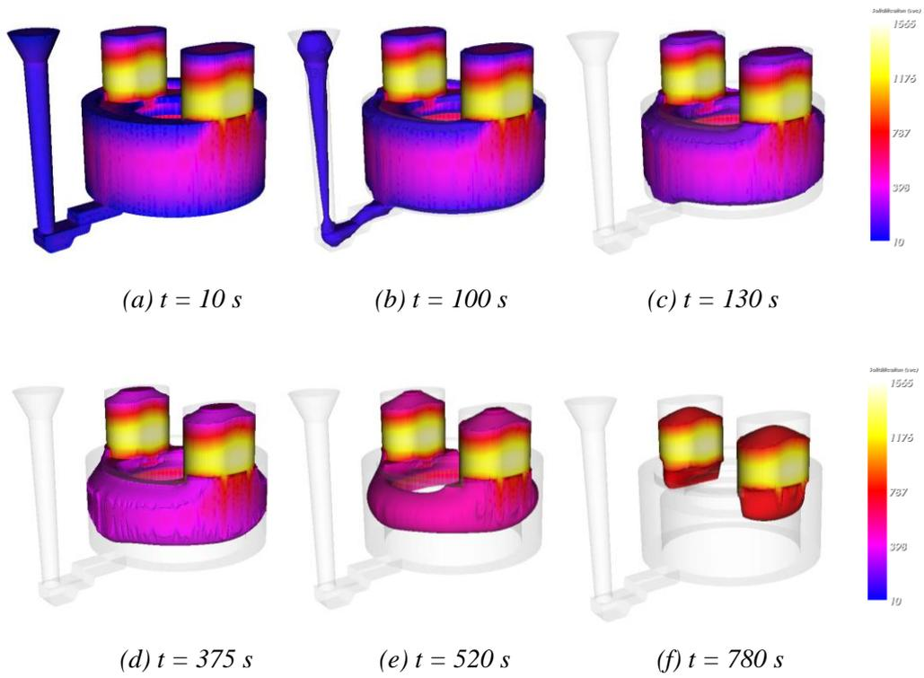
Figure 10. The solidification process of optimized scheme II.
