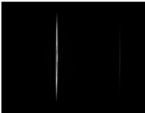
Figure 4. PEN – light, Hg I, 435 nm, ICCD camera, a. integral profile - picture from program SpectraSuits, b. Integral profile – after data processing in Origin.
