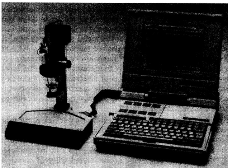
Figure 3. The multi-purpose pen-type RME in the polarographic stand, connected to a lap-top PC unit.
