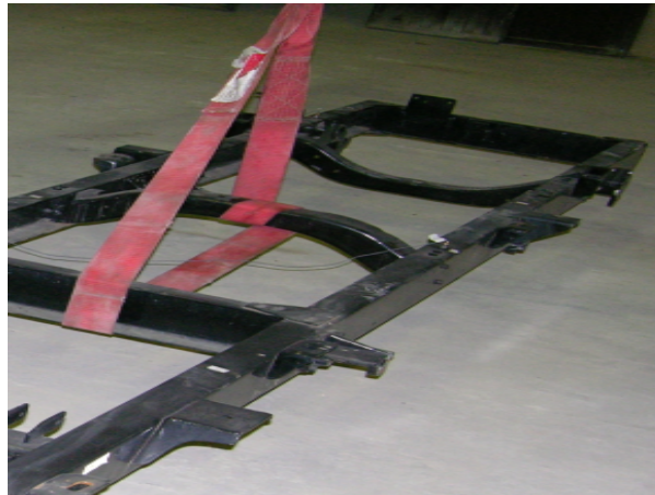
Fig. 6 Experimental modal test (suspended by a hook)
