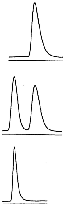
Figure 2. HPLC analyses of trans -1,2-diphenylcyclopropanes on a triacetylcellulose column; top, (+)-(1 S ,2 S )-1- d 0 , retention time 65.5 min; middle, rac -1- d 0 ; bottom, (-)-(1 R ,2 R )-1- d 2 , retention time 49.5 min.
