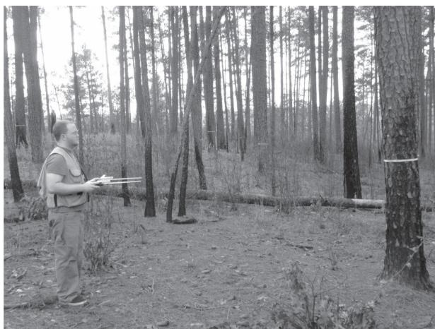
**Fig. 2** Remote measurements conducted with the laser caliper dendrometer
