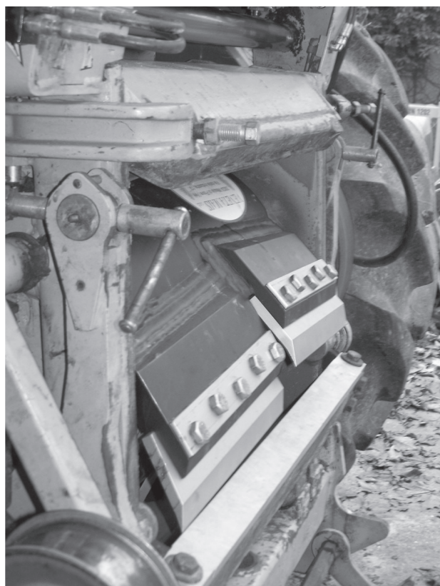
Fig. 1 Experimental drum mounted on self propelled chipper Claas Jaguar 890
