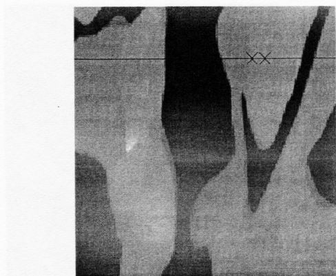
Figure 12. A 5\ \mu\text{m} \times 5\ \mu\text{m} SFM image and height profile along the indicated line of HO-(CH 2 ) 24 -OH crystal-lites on freshly cleaved mica; a step of monolayer thickness is given by the vertical arrow in the profile.
