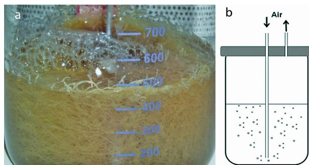
**Fig. 5.** Mass proliferation of hairy roots cultured in an airlift bioreactor (a) and schematic representation of the airlift bioreactor (b)
