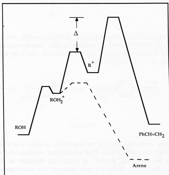
Figure 1. Free energy profiles for dehydration reactions: (—)  $\alpha$ -phenylethanol; (---) hypothetical concerted mechanism for arene hydrate.
