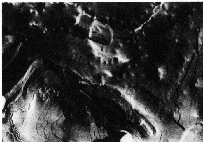
Figure 7. TEM micrograph of MgDBS lamellar phase (equimolar \text{Mg}(\text{NO}_3)_2 and HDDBS of 6 \times 10^{-2} mol \text{dm}^{-3} ; total magnification 53000x. The bending of the lamellar multilayers into a globular form can be clearly seen in the lower right part. The sinusoidal trace in the left part shows the previously existing spherulites. Some round traces have also remained from the individual spherulitic positions (the upper right part).
