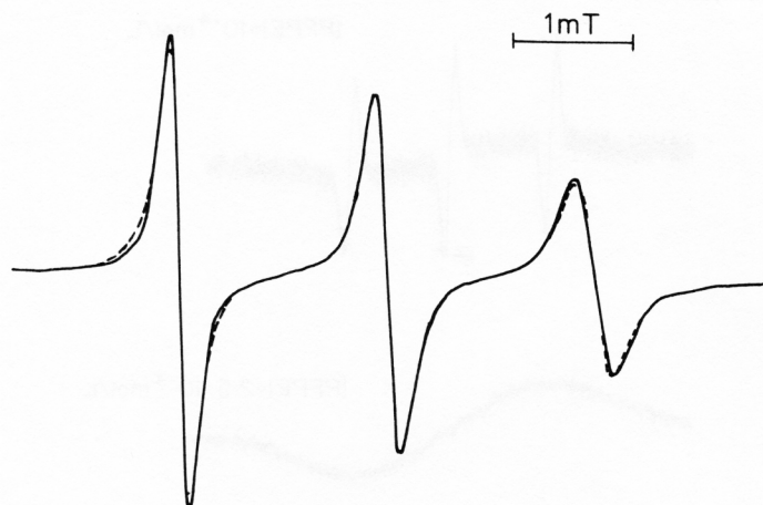
Figure 10. Experimental spectrum ( T = 293 K) for TempTMA + 2 \times 10^{-5} mol/L in a 2 \times 10^{-3} mol/L PFPE solution (full line). For the computed line, see text.
