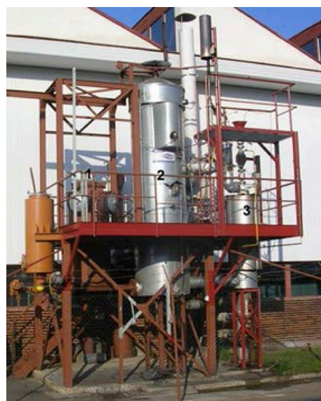
Fig. 1 – Atmospheric fluidized bed gasifier Biofluid 100
