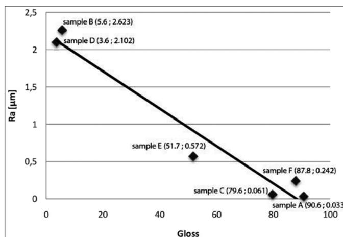
Figure 2: Correlation between surface roughness (Ra) and surface gloss
