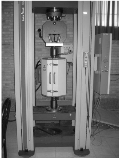
Fig. 4 Pressure test device and the furnace
