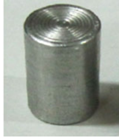
Fig. 6 Cylinder pressure test specimen
