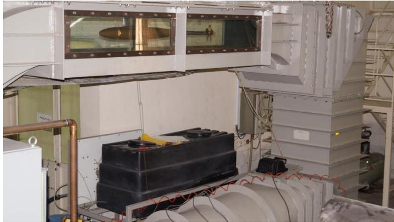
Fig. 3 Test section K23 cavitation tunnel
