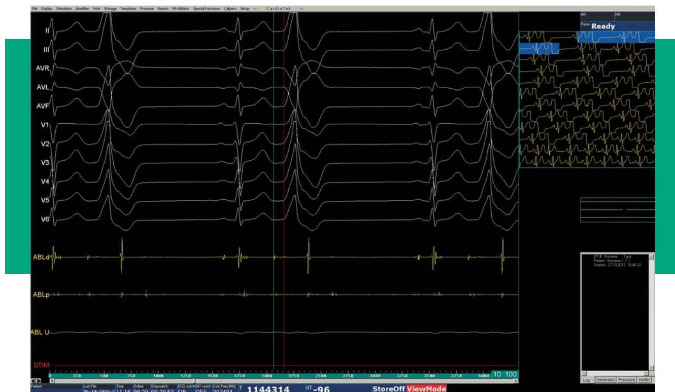
Figure 5. Signals from the ablation catheter positioned at the left aortic cusp (same patient as at Figure 4 ). Upper panel shows 12-lead electrocardiogram, ABLd-bipolar electrogram from the distal part of the tip of the catheter, ABLp-bipolar electrogram from the proximal part of the catheter's tip, ABL U-unipolar electrogram from the ablation catheter. During premature ventricular complex, discreet, sharp potential is reproducibly registered that precedes QRS by 96 ms. This signal represents isolated myocardial fiber potential and stems out of myocardial extension into aorta thus the designation-great arterial potential. During sinus QRS complexes this signal comes after the local ventricular electrogram, pattern is reversed during premature ventricular complex.
