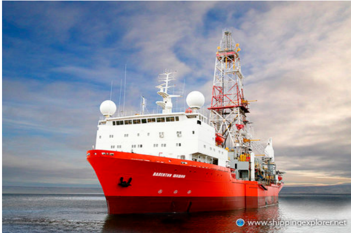
Figure 1. Drillship with derrick
