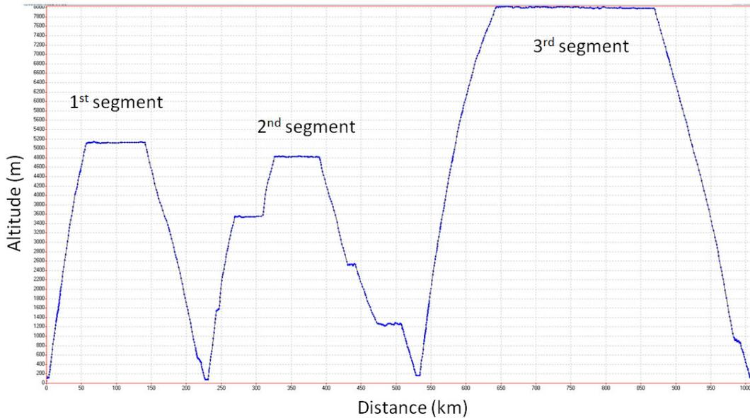
**Fig. 1** Example of a vertical profile of a three-segment navigation route (test flight 3) based on GPS measurements of the flight altitude and ground speed.
