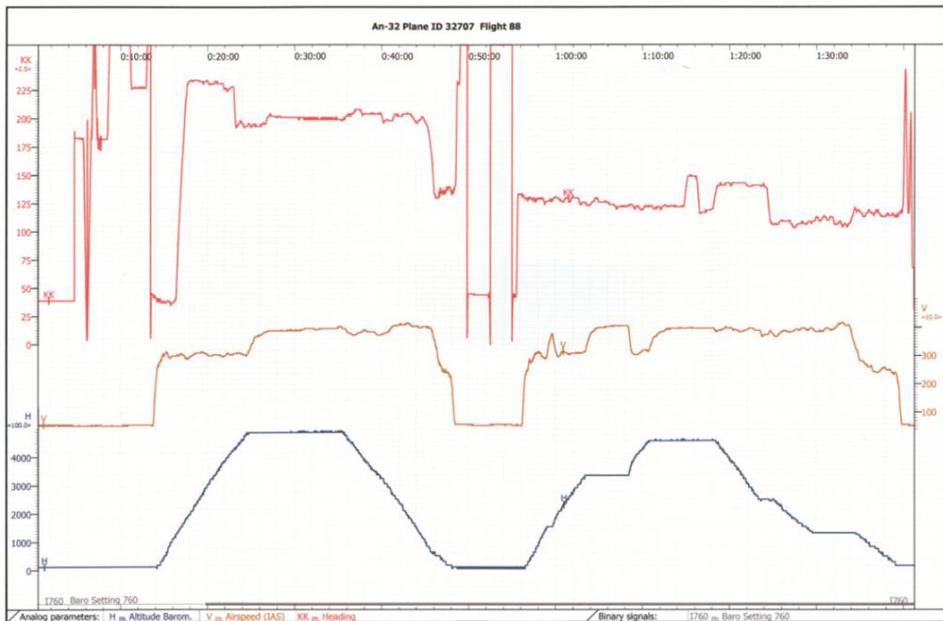
**Fig. 2** Data log of CAS and flight altitude recorded by on-board BUR-4-1-05 sensors
