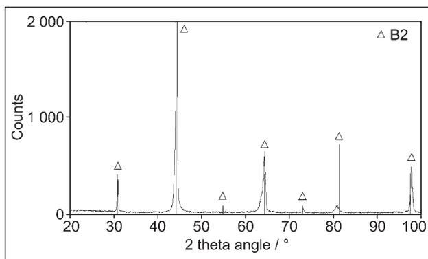
**Figure 1** Diffraction pattern of FeAl28Cr5 alloy after heat treatment at temperature 900 °C for 24 h
