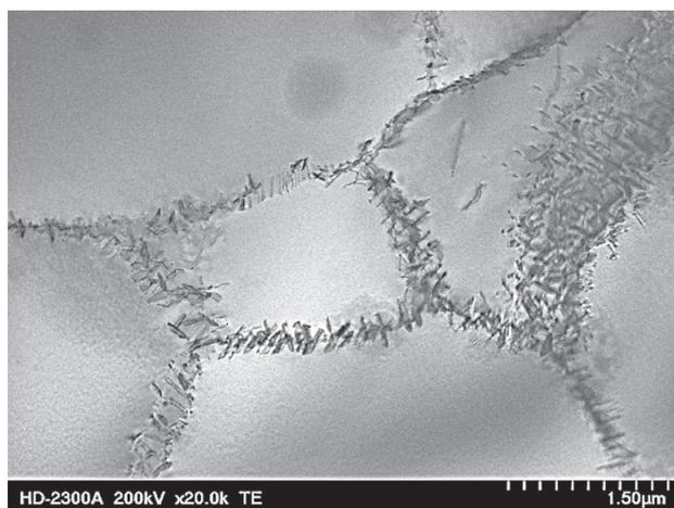
**Figure 11** Substructure of FeAl28Cr5 alloy after hot rolling process. Secondary phases around the grains / subgrains
