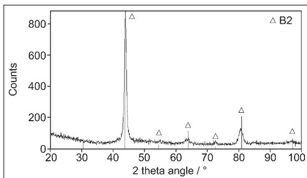
**Figure 2** Diffraction pattern of FeAl38 alloy after heat treatment at temperature 900 °C for 24 h
