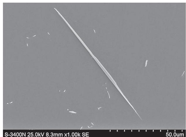
**Figure 4** Microstructure FeAl38 of after annealing at temperature 900 °C for 24 h - SEM, phases elongated in shape
