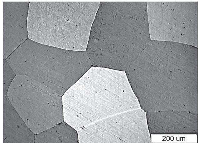
**Figure 8** Microstructure of FeAl38 alloy after hot rolling process
