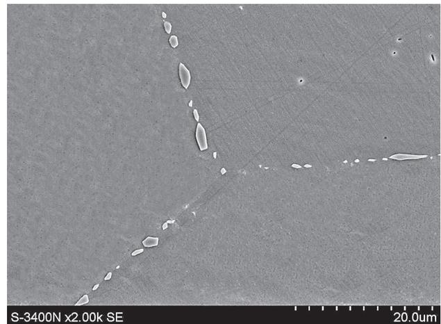
**Figure 3** Microstructure FeAl28Cr5 of after annealing at temperature 900 °C for 24 h - SEM, phases on the grains boundaries
