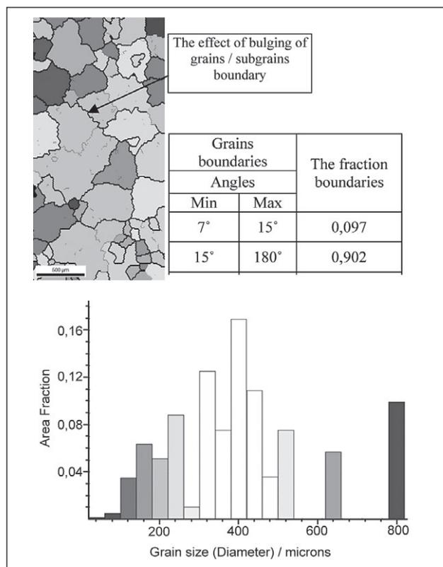
**Figure 10** EBSD map, boundaries incidence and grain size distribution for FeAl38 after heat treatment and hot rolling
