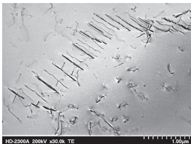
**Figure 12** Substructure of FeAl38 alloy after hot rolling process. Dislocations and secondary phases
