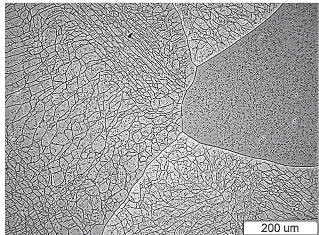
**Figure 7** Microstructure of FeAl28Cr5 alloy after hot rolling process
