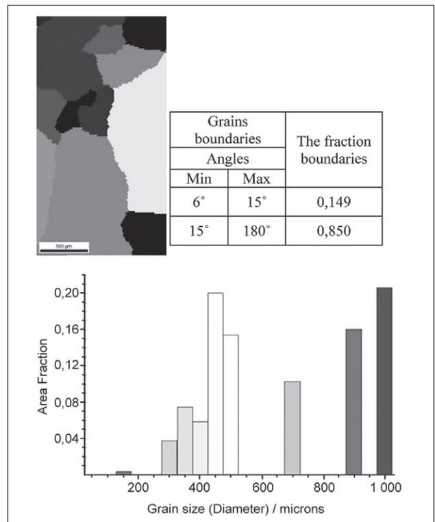
**Figure 9** EBSD map, boundaries incidence and grain size distribution for FeAl28Cr5 after heat treatment and hot rolling
