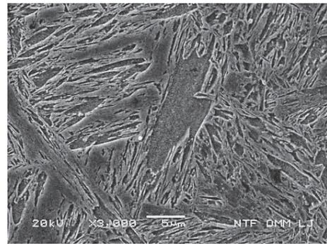
Figure 1 The microstructure of steel PROTAC 500 (SEM)
