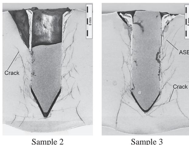
Figure 4 Macroscopic picture of breakthroughs bullets through the samples 2 and 3, marked as cracks and ASB
