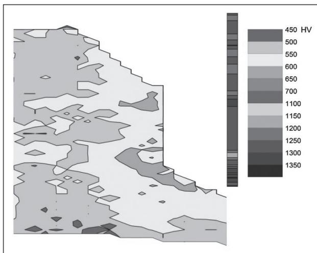
**Figure 6** Distribution of hardness of the steel in the vicinity of the bullet penetration through sample 3
