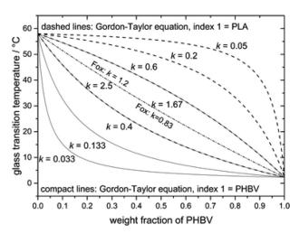
Fig. 3 – Gordon-Taylor equation for PLA ( $T_g = 58$  °C) and PBHV ( $T_g = 2.5$  °C) with index 1 for PLA (dashed lines) or PHBV (full lines) and different k-values
