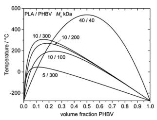
Fig. 2 – Spinodal curves for binary blends of PLA and PHBV using a solubility parameter difference of  $\Delta\delta=0.65~J^{0.5}$  cm<sup>-1.5</sup> and density of both polymers of  $\rho=1.25~g~cm^{-3}$ ; molecular weights (kDa) are presented at the curves
