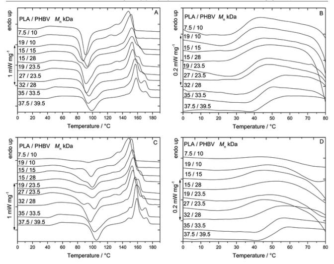
Fig. 4 – DSC Thermograms of PLA / PHBV Blends (80:20), 4a and 4b: melt (190 °C) quenched samples (liquid nitrogen), 4c and 4d: samples with controlled cooling (20 K min<sup>-1</sup>) from the melt; molecular weights are presented at the curves, which are shifted for better visualisation; double arrow indicates scale of heat flow.
