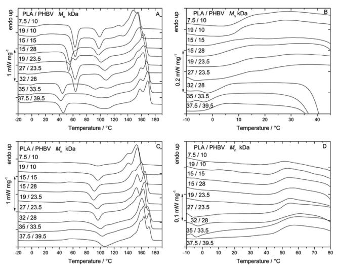
Fig. 7 – DSC Thermograms of PLA: PHBV Blends (50:50), 7a and 7: melt (190 °C) quenched samples (liquid nitrogen), 7c and 7d: samples with controlled cooling (20 K min<sup>-1</sup>) from the melt; molecular weights (kDa) are presented at the curves which are shifted for better visualisation; double arrow indicates scale of heat flow
