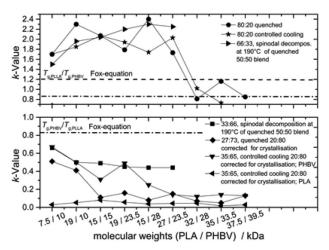
Fig. 5 – k-Values derived from G-T-equation for 80:20, 50:50 and 20:80 blends of PLA and PHBV; (eq. 6; see also Fig. 3 for explanation); 80:20 control cooling with PLA/PHBV = 37.5/39.5: k = 0.5
