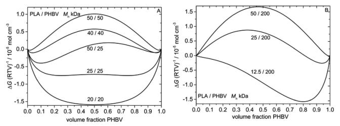
Fig. 1 – Free enthalpy of mixing at 190 °C of PLA and PHBV according to Flory-Huggins theory and a difference in solubility parameter of 0.65  $J^{0.5}$  cm<sup>-1.5</sup> and density of both polymers of  $\rho = 1.25$  g cm<sup>-3</sup> in dependence of molecular weight (kDa, figures at the curves); a: general influence, b: influence of low molecular weight components
