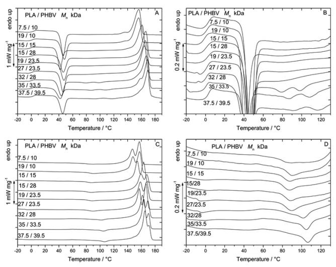
Fig. 6 – DSC Thermograms of PLA: PHBV Blends (20:80), 6a and 6b: melt (190 °C) quenched samples (liquid nitrogen), 6c and 6d: samples with controlled cooling (20 K min<sup>-1</sup>) from the melt; molecular weights (kDa) are presented at the curves, which are shifted for better visualisation; double arrow indicates scale of heat flow
