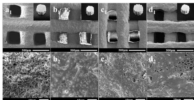
Fig. 6 – SEM images of composite scaffolds of P(HB-HHx) and mesoporous bioactive glass (MBG) at different magnifications (top and bottom). A: reference material poly(vinyl alcohol):MBG = 1:7; B: P(HB-HHx):MBG = 1:7; C: P(HB-HHx):MBG = 1:5; D: P(HB-HHx):MBG = 1:3. Reproduced in part from reference<sup>95</sup> with permission of The Royal Society of Chemistry.
