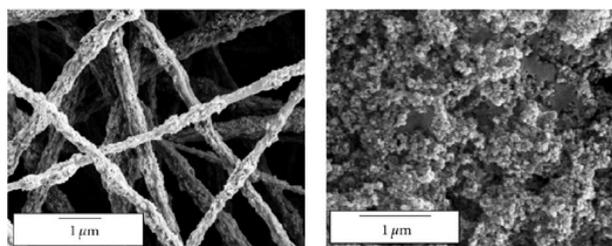
Fig. 5 – SEM micrographs showing the morphological features of electrospun fibers (left) and spincast films (right) of PHB blended with TiO<sub>2</sub>. Reprinted from reference<sup>75</sup> with permission from Hindawi Publishing Corporation.
