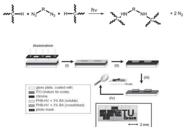
Fig. 3 – Top: Crosslinking of polymer chains with a bisazide (BA) under UV irradiation. Bottom: Multi-step photolithographic processes based on P(HB-HV). Reproduced in part from reference<sup>14</sup> with permission of The Royal Society of Chemistry.
