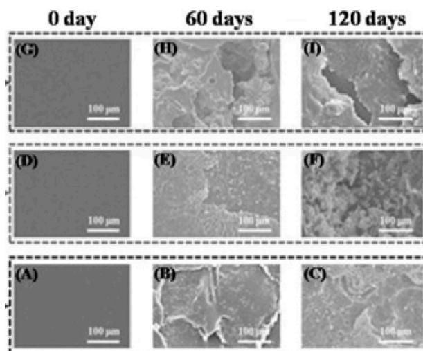
Fig. 4 – SEM images of the morphology of PHA composites after 0, 60, and 120 days of degradation. A-C: pristine PHA, D-F: PHA crosslinked with cellulose acetate, G-I: PHA grafted on acrylic acid/cellulose acetate. Biodegradation by *Acetobacter pasteurianus* can be monitored by the erosion in the films. Reprinted from reference<sup>66</sup> with permission from Elsevier.
