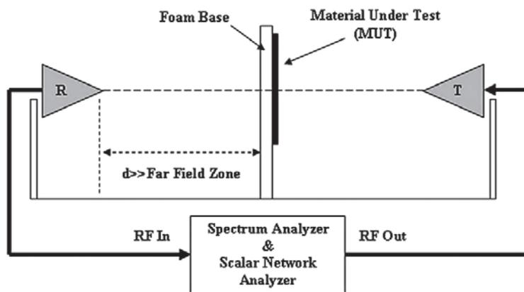
Fig.4 The measurement set-up [19]
