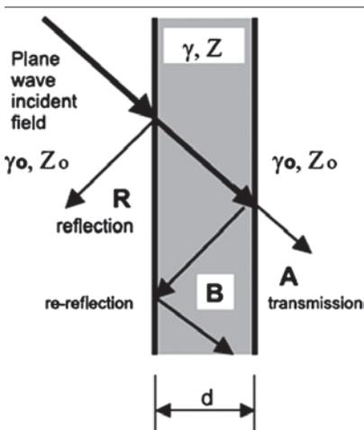
Fig.1 Wave transmission on a thin layer of media [14]
