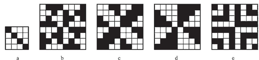
Fig.2 Weave patterns used in experimental: a - 1/3 twill; b - Diced weave 1; c - Diced weave 2; d - Diced weave 3; e - Diced weave 4
