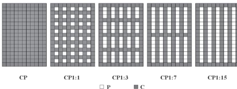
Fig.3 Schematic diagram of open-grid structures formed in the woven fabrics (gray squares: conductive core yarns; white squares: polyester yarns)
