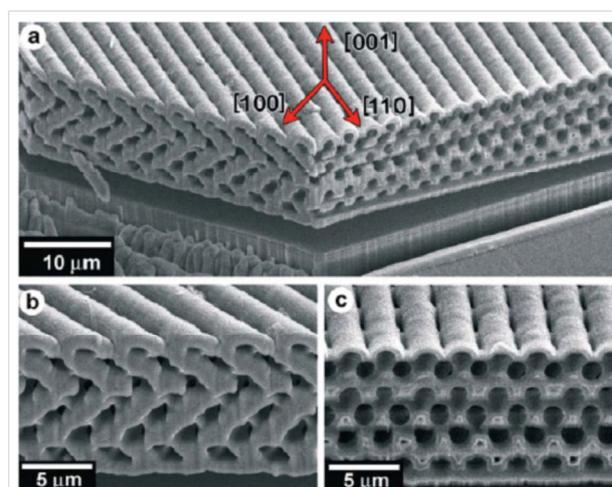
**Figure 8.** Scanning electron microscopy views of a germanium photonic crystal with a diamond-based woodpile structure. The sample was fabricated by the direct ink writing of a template followed by chemical vapour deposition of germanium. This structure has a complete photonic band gap in the infrared region of the electromagnetic spectrum. Adapted from reference [24]. Copyright Wiley-VCH Verlag GmbH & Co. KGaA. Reproduced with permission.
