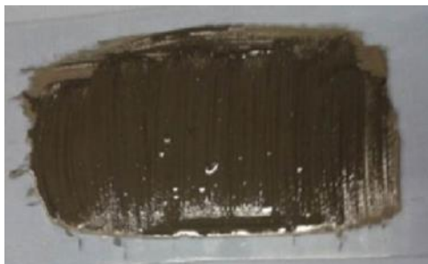
Figure 5. Adhesion of Carbo e-Therm on PET film
