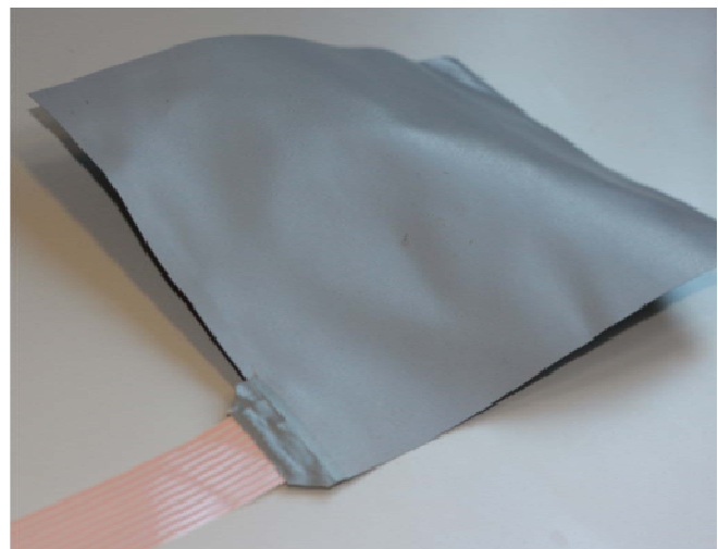
Figure 4. a) Conceptual design of IMAT standard heater IMAT-S; b) IMAT-S prototype
