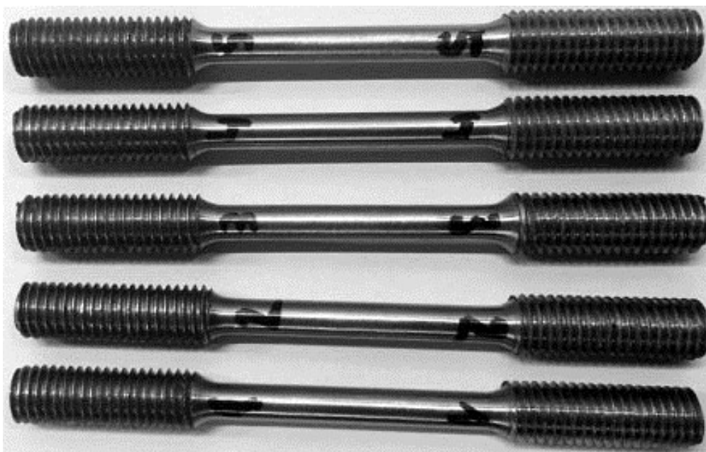
Figure 5. Specimens for static tensile test.
