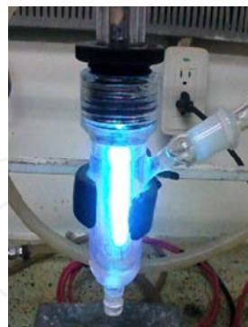
Figure 1. Photochemical reactor for the synthesis of the bioconjugate FA-AuNP
