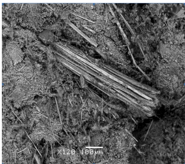
Figure 3 Chrysotile fibres on electronic microscope (magnification 120x)
