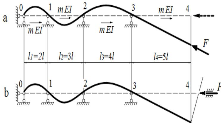
Figure 2. Continuous beam loaded with non-conservative forces
