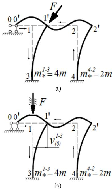
**Figure 3.** Plane frame: a) force of  $F$  follows up the assembly rotation angle 1; b) force of  $F$  has a fixed action line.
