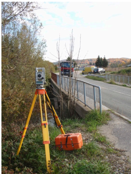
Fig. 8. Total station 1 on the Pernica Bridge. Fig. 9. Total station 2 on the Pernica Bridge.
