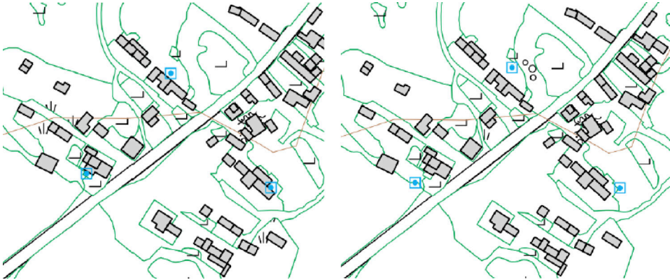
Fig. 2. Representation of objects from “WaterChamber” class (left) and after the shift (right).
