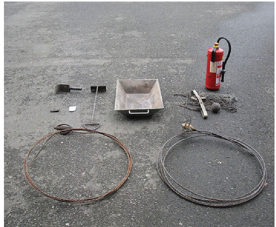
Figure 4: Equipment and means for extinguishing chimney fires
