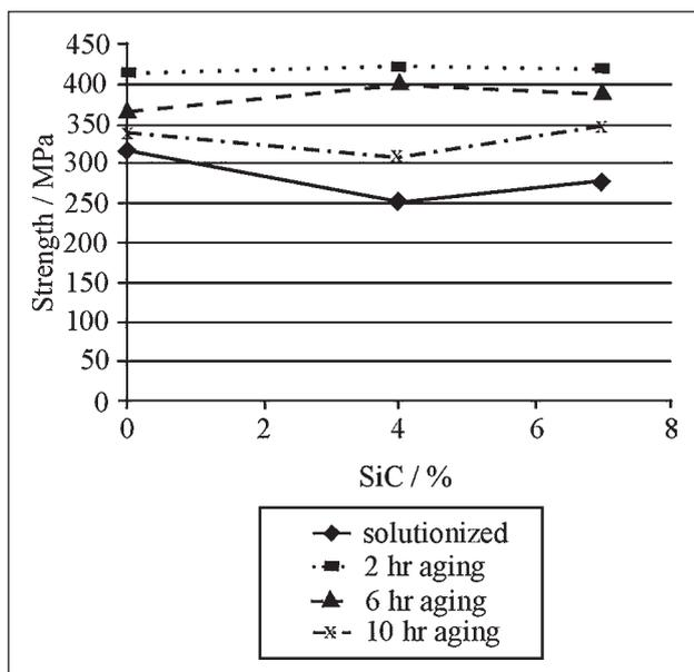
Figure 4 Relationship between strength and SiC content with increasing in aging time
