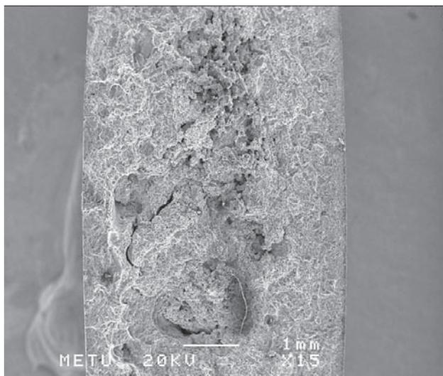
**Figure 7** Fracture surface of tested specimen with high porosity and cavities
