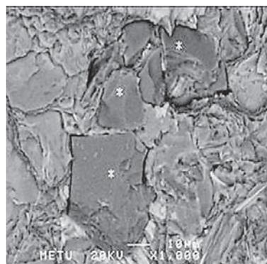
Figure 6 SEM photograph of SiC particles (Magnification 1 000 X)
