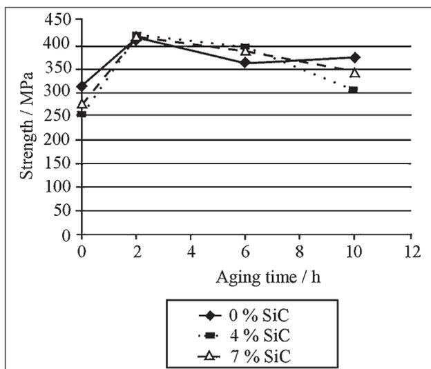
Figure 5 Flexure strength related to aging time with different SiC contents
