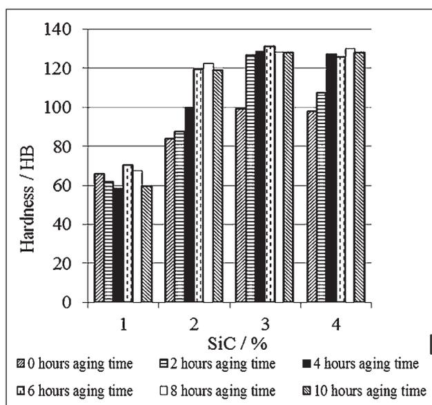
Figure 2 Effect of aging time and SiC content on the hardness behaviour (1) Matrix, (2) Matrix with 1,5% Mg, (3) Matrix with 1,5 % Mg and 4 % SiC, (4) Matrix with 1,5 % Mg and 7 % SiC
