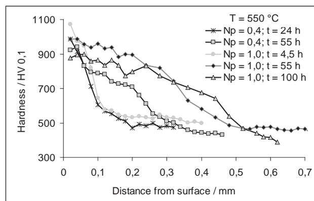
**Figure 4** Hardness distribution in die segments nitrided using the ZeroFlow method at various parameters of the 2<sup>nd</sup> process step (1<sup>st</sup> step parameters:  $T = 490$  °C,  $N_p = 15$  atm<sup>-1/2</sup>,  $t = 1$  h)
