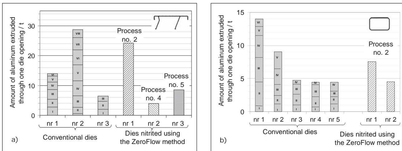
**Figure 5** Operating life of dies nitrided conventionally and nitrided using the ZeroFlow method: a) flat, b) hole (successive nitriding regeneration processes were marked by Roman numerals I-VIII on the bars of conventionally nitrided dies)
