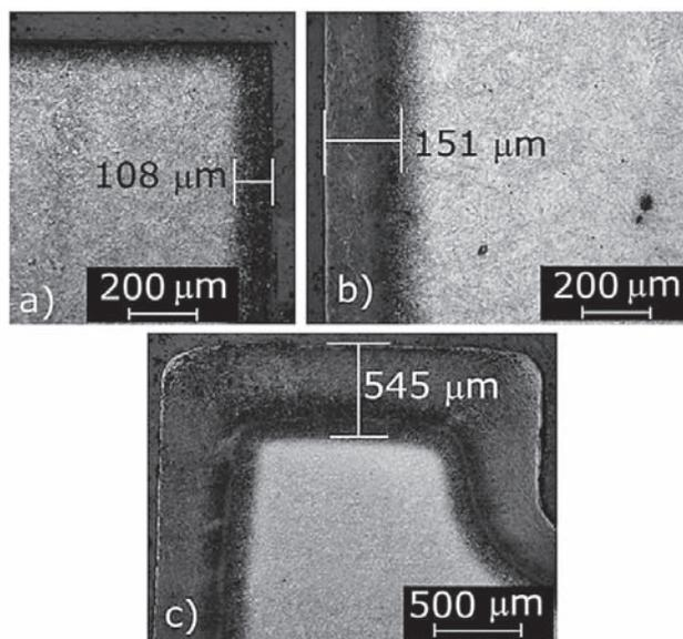
Figure 2 Structure of bearing of die after different numbers of nitriding regeneration cycles: a) 1<sup>st</sup> nitriding, b) 3<sup>rd</sup> nitriding, c) 8<sup>th</sup> nitriding, exploited until worn out
