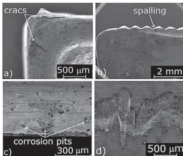
Figure 1 Examples of wear of the bearing surface of dies
