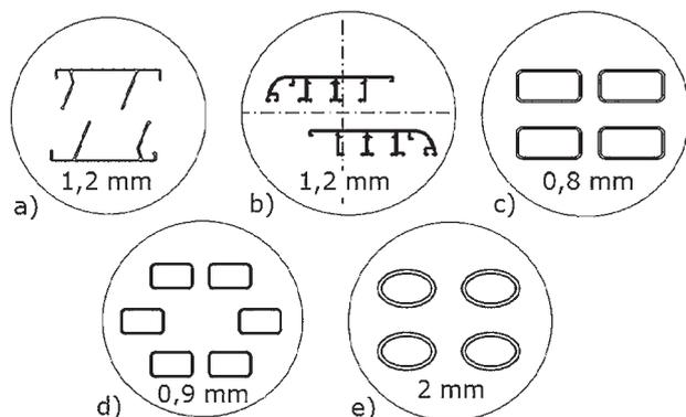
**Figure 3** Shapes of dies for extruding aluminum profiles and wall thicknesses of the profiles extruded through them
