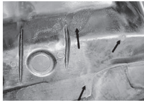
Figure 2 Mold erosion wear [7]
