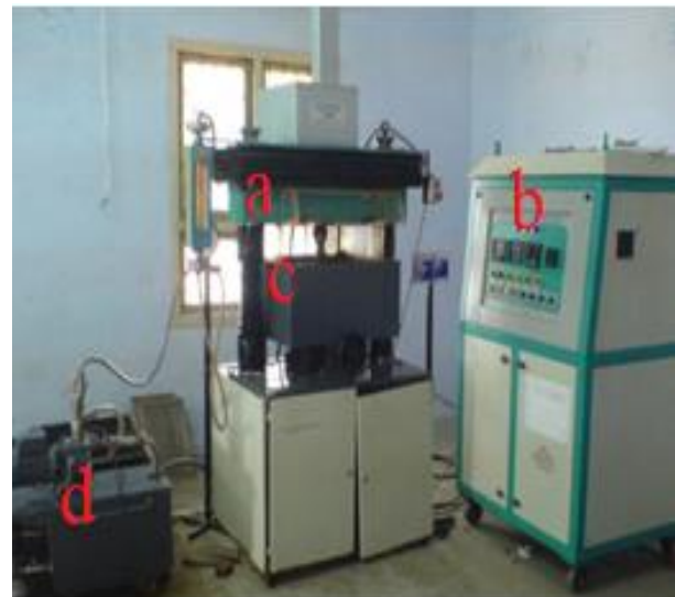
Figure 2. Experimental set up of ECM: a) Total feed system, b) Control panel, c) Machinery chamber, d) Electrolyte tank.
