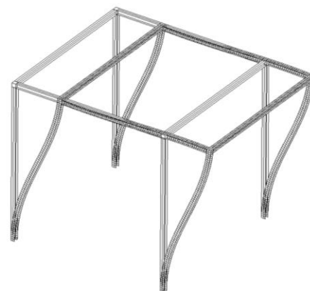
Figure 7. Sway buckling mode – shell model NASTRAN.
