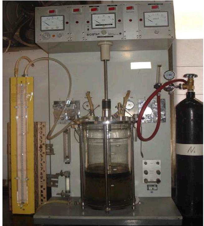
Fig. 1 – Lab-scale TLPPB used for crude oil removal
