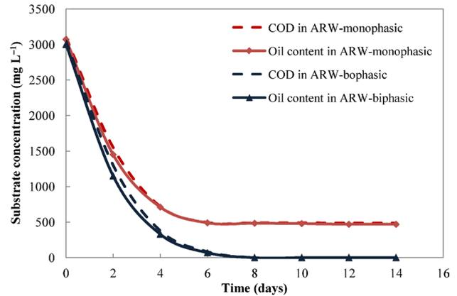
Fig. 5 – Profiles of substrate removal in actually contaminated river-water (ARW) samples in monophasic and biphasic bioreactors
