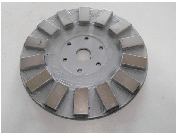
Figure 4 The Rotor Structure of TAFPMOS-NN Type Motor [21]
