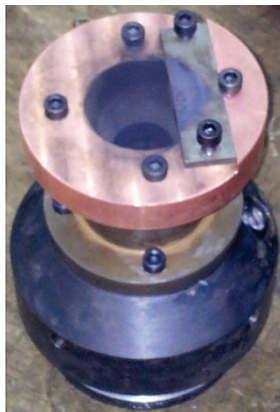
Figure 13 Nozzle after test with tab blocking 20 % of exist area
