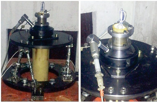
Figure 11 Rocket motor on test stand before firing
