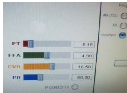
Fig.4. Case study parameters – pantoscopic tilt is in the minus range (measured with »Impression Integrated Service Terminal«).
