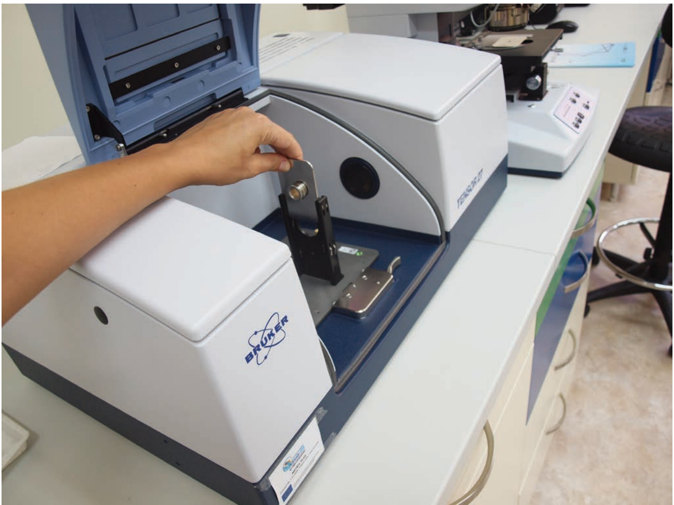
Sl. 3 Postavljanje stalka s pastilom za analizu u IR spektrometar (snimila T. Zubin Ferri) Fig. 3 Putting the stand with the pastille to be analyzed in the infrared spectrometer (photo by T. Zubin Ferri)
