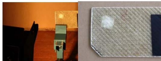
**Figure 10** Impacted specimen
