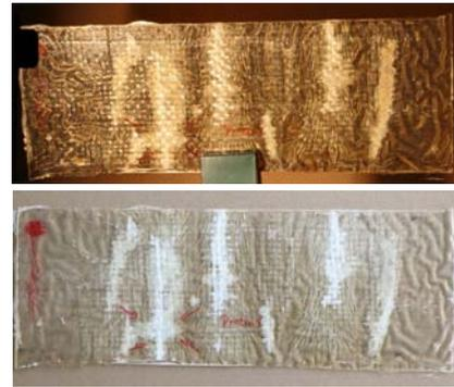
**Figure 15** Impacted and severely delaminated specimen
