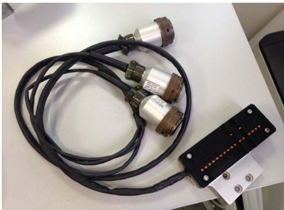
Figure 10 HRID matrix eddy current probe for inspection of sealing surfaces
