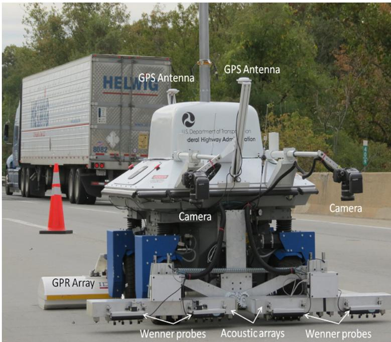
**Figure 4** Front end of RABIT with NDE and navigation components.
