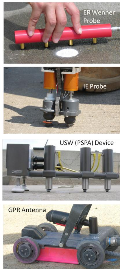
**Figure 3** Samples of probes and devices of NDE technologies implemented in RABIT.
