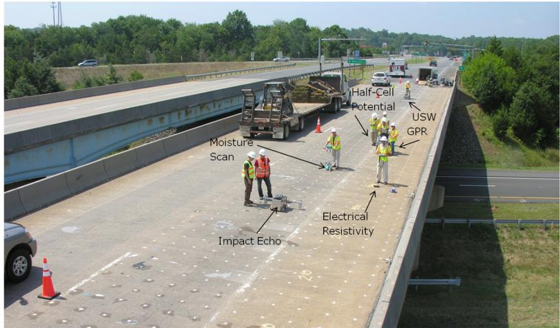
**Figure 2** Most commonly used NDE technologies in detection of corrosion induced deterioration.
