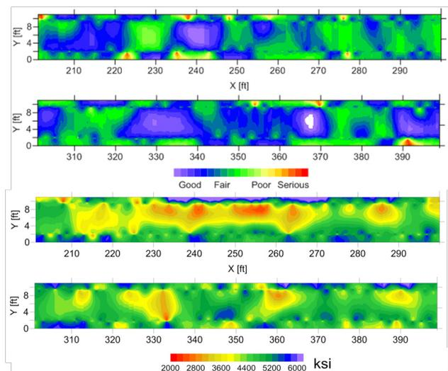
**Figure 6** Delamination map (top) and concrete modulus map (bottom).
