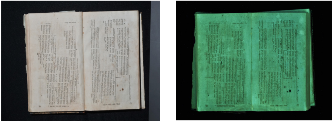
Figure 5. Folios 762v-763r in Scriptores rerum Hungaricarum veteres ac genuini . Foxing stains in early stage: slightly brown coloured stains, and slightly visible (left), but clearly distinguishable under UV-light (right).
