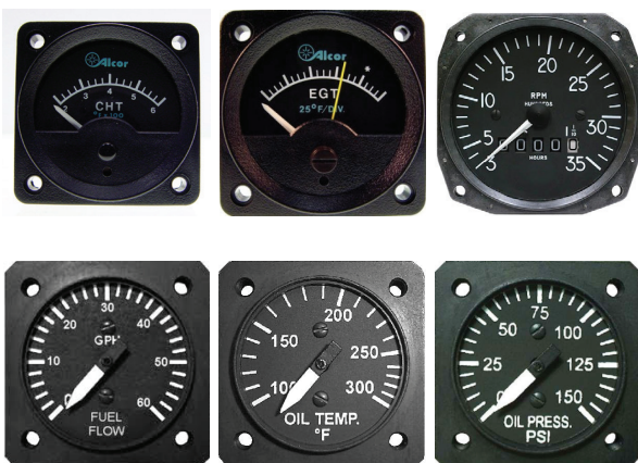
Figure 1 Classical gauges for monitoring of aircraft piston engine (CHT, EGT, RPM - rotation speed, FF - fuel flow, oil temperature and oil pressure)
