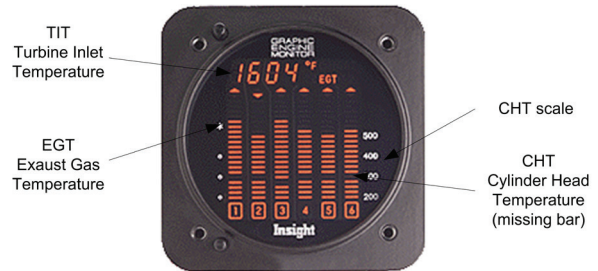
Figure 5 Engine monitor with bar graph display (Insight Avionics, older GEM 603)
