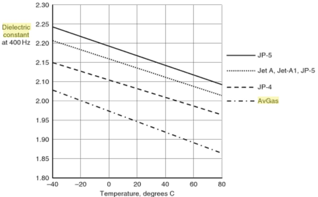
**Figure 1** Dielectric constant vs. temperature for typical aircraft fuel at 400 Hz (adopted from [2])
