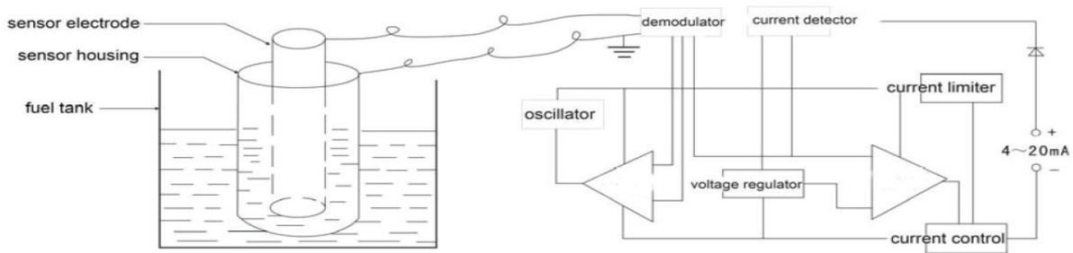
**Figure 2** Fuel level sensor schematic
