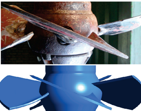
Figure 1 Compatibility of actual blade with modelled geometry
